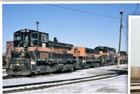
IHB 9206 is positioned at the Blue Island Ready Track during winter 2001. It was built in 1966 by General Motors' Electro-Motive Division at its La Grange, Ill., facility.
